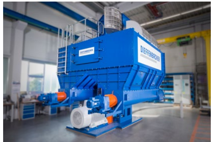
Flameless explosion venting in a grinder machine.
